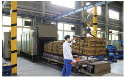
台车式热风循环炉 Trolley-type Hot Air Circulating Furnace
